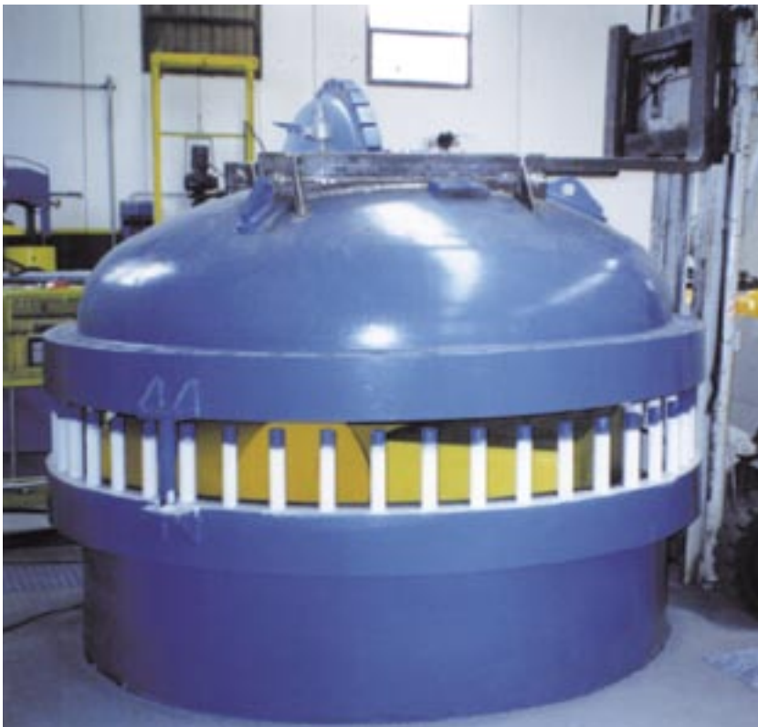
Pressure tanks for high depth tests
